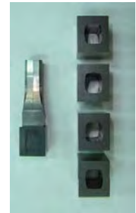
(a) Piercing die set (b) punch & dies Fig. 1 Piercing punch & dies for piercing of the lead frame
