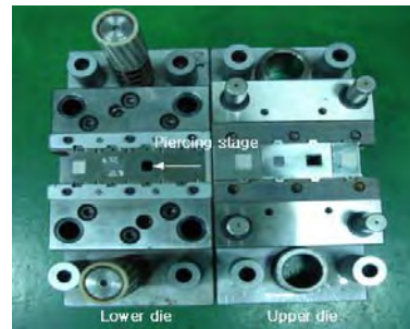
(a) Piercing die set (b) punch & dies Fig. 1 Piercing punch & dies for piercing of the lead frame
