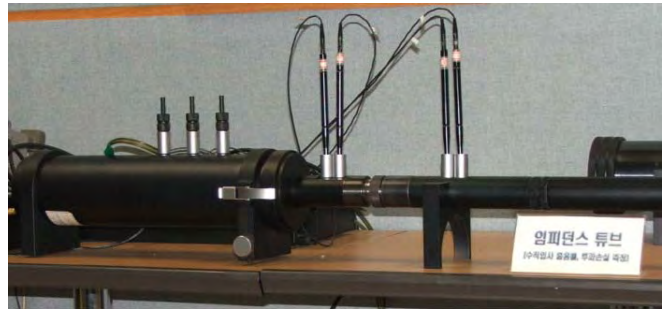
Fig 2. Impedance tube type measuring instrument
