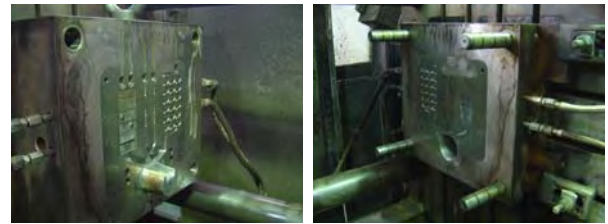
(a) Moved side (b) Fixed side
