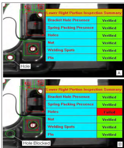
Fig. 2 MVIS Sample Test Results: (a) GQRT for lower right portion all returning "VERIFIED", (b) MPRT sample for lower right portion of the car seat bottom cushion frame.
