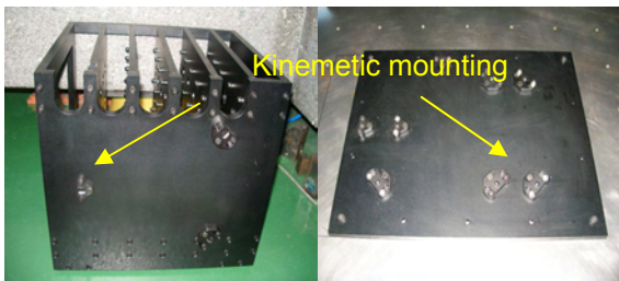
Figure 2: 3-D artifact and its kinematic mounting base.
