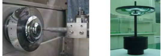
Fig. 3 Machining reflector mirror by SPDTM and prototype
