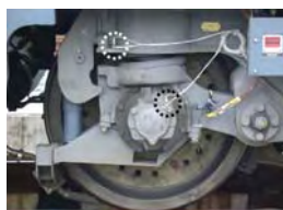
Figure 1 Axel box and Accelerometer mounted on bogie frame
