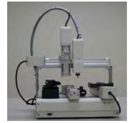
Fig. 8 Lens assembly cell
