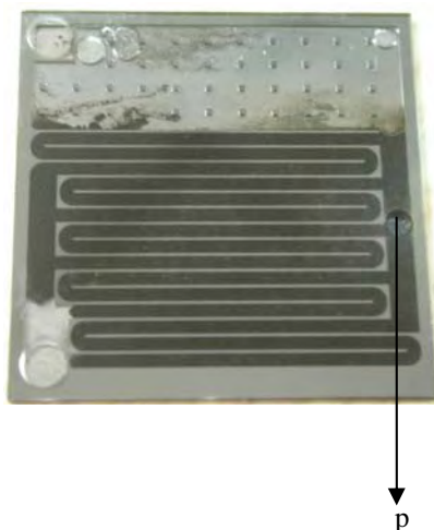
Figure 2. Catalyst loaded MEMS reactor
