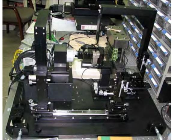
Fig.1 Dynamic micro material property measurement system
