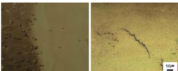
Fig. 5 Laser cladding with IN 625 powder(L) and IN 939 powder(R) 634
