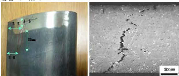
Fig. 4 Crack for welded blade with GTD 111 at 1,100°C
