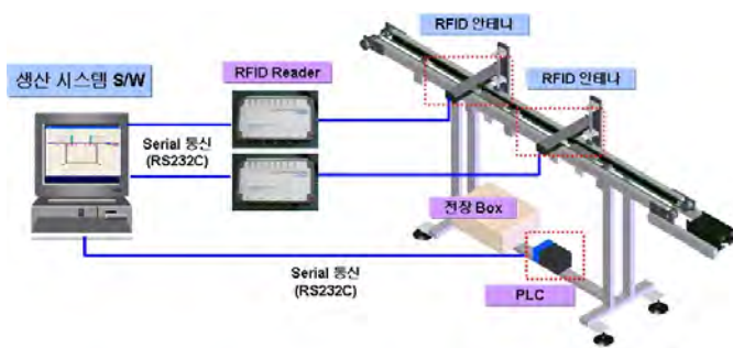
Fig. 2 Schematic Diagram of Test-bed using RFID system
