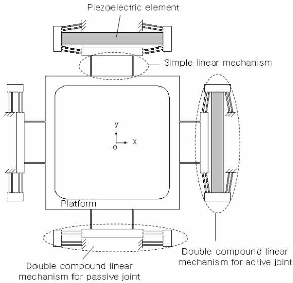
Fig. 2 The structure of ultra precision stage implemented by 4-PP compliant mechanism
