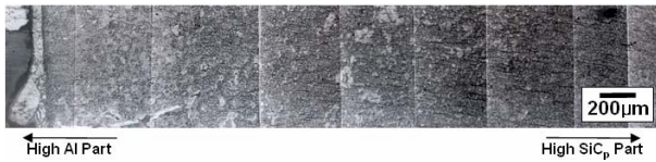
Fig. 1. Microstructures of gradient layer of Al-SiC p FGM with thickness of 3mm
