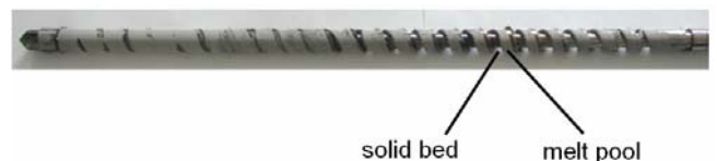
Fig. 2. Screw with molten feedstock fraction
