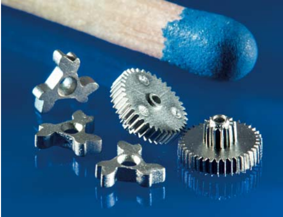
Fig. 2. Stainless steel \mu -MIM parts (Scholz GmbH)
