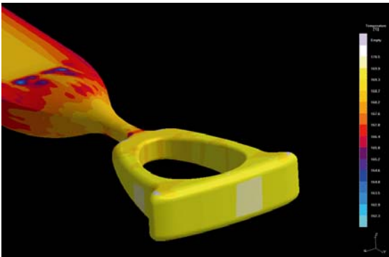
Fig. 3. 3D-simulation of temperature distribution after mould filling
