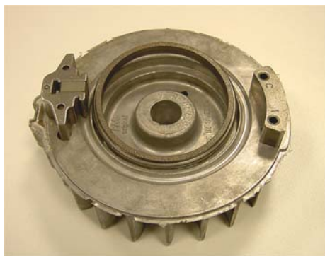
Fig. 1. Magnet part to the left and balance weight part to the right.
