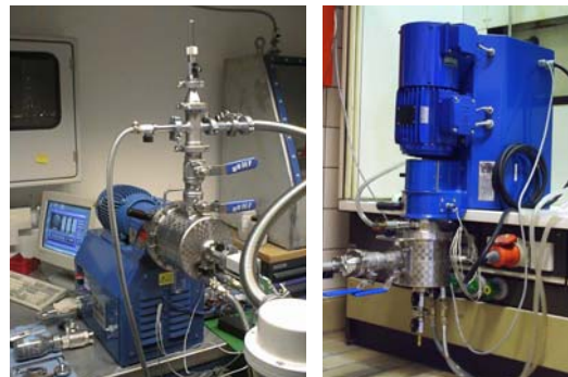
Fig. 1(left): horizontal rotary ball mill (Simoloyer® CM01-21) with air-lock for loading, operation and unloading under vacuum and/or inert-gas.
