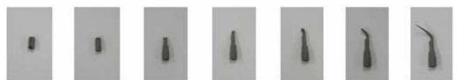
Fig. 8. Short shot experiment of dental scaler tip using PIM feedstock with STS316L.
