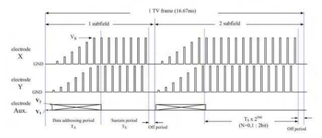
Figure 4: Drive waveforms for the areal selective 2-bit dimming
