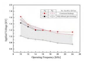
Figure 2: Operating voltage margin
