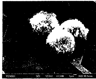
Fig. 2. A SEM image for magnetic beads (SPHERO™ SVM series) on a spin-valve device
