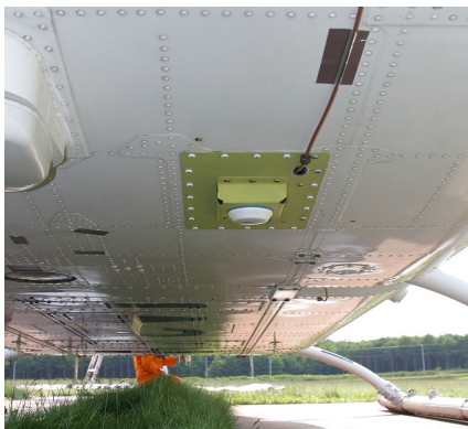
Figure 9 Pseudolite antenna underneath the helicopter
