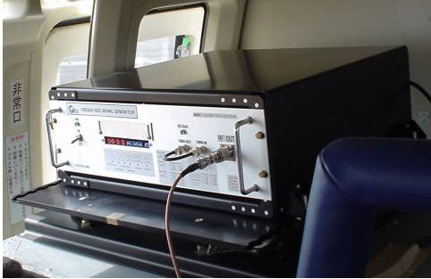
Figure 8 JAXA's experimental helicopter MuPAL-e and pseudolite installed in the cabin
