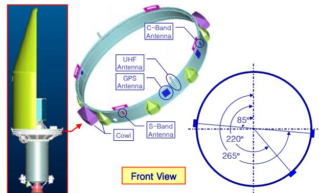
Figure 1. Placement of the GPS Antennas on KSLV-I.
