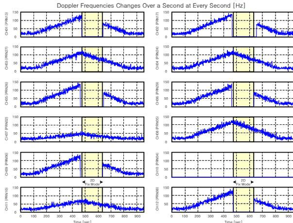
Figure 10. Changes of the Doppler Frequency Shift Over a Second at Every Second.
