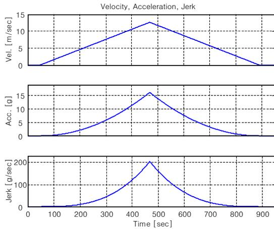
Figure 5. Velocity, Acceleration and Jerk in the Scenario.
