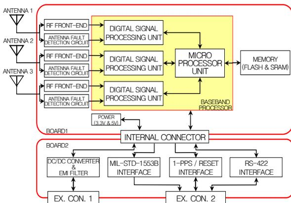
Figure 2. GPS Receiver for Satellite Launch Vehicle.
