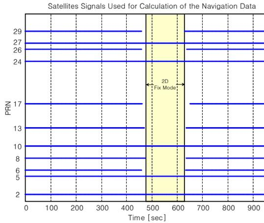
Figure 8. Satellite Signals Used for Calculation of Navigation Data.
