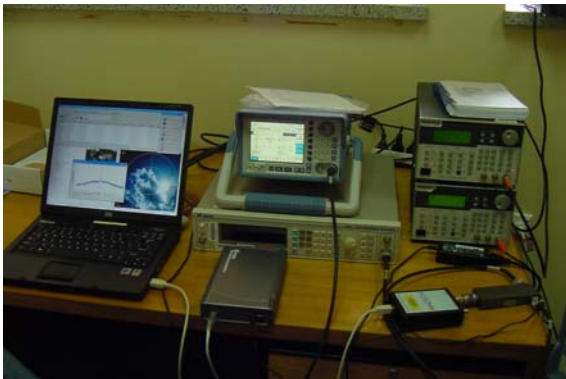
Figure 4 NordNav software receiver and the RF signal generators to generate swept CW RFI
