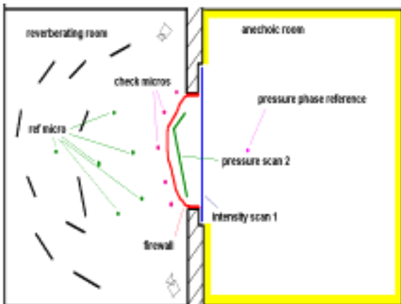
Fig.7 Buck test setup
