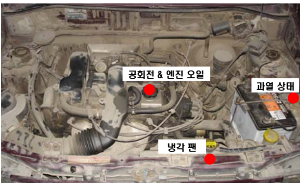
Fig. 1 The location of sensors for measurement of the engine signal
