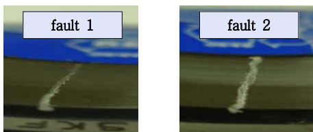
Fig.3 fault of bearing outer race
