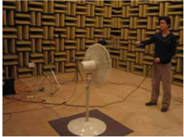
Figure 3. Measurement of the sound power level by intensity method
