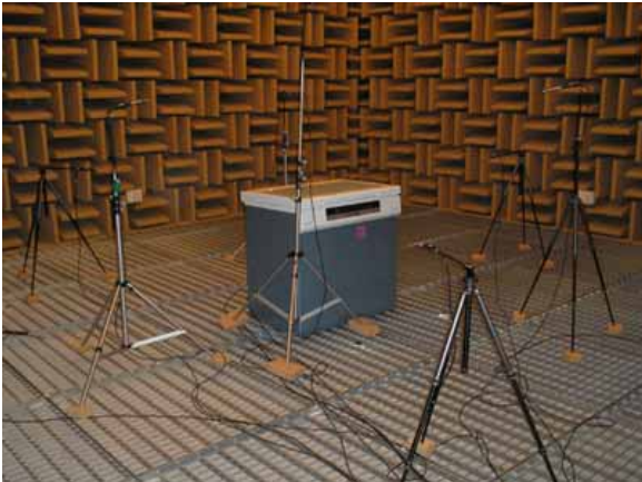
Figure 1. Measurement of the sound power level in the semi-anechoic room.
