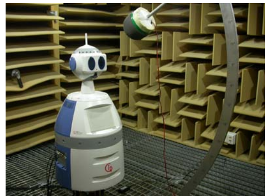
Fig. 4 Experimental setup in anechoic chamber; adapted form [8]
