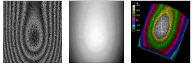
Fig. 6 Phase map, Unwrapping, 3DPolt (+0.4mA, 5.5 μ m)
