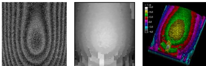
Fig. 5 Phase map, Unwrapping, 3DPolt (+0.2mA, 5.5 μ m)
