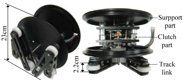
Fig. 6 Prototype of selectable wheel-track mechanism
