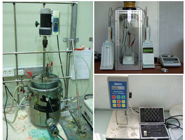
Fig. 2 Small-sized stirrer, NCO and viscosity measuring devices
