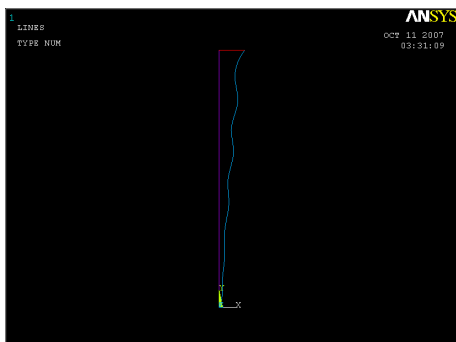
Fig. 3 Unfeasible shape of microneedle for mold process
