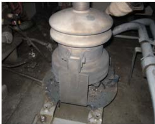
(a) DC arrester dielectric breakdown
