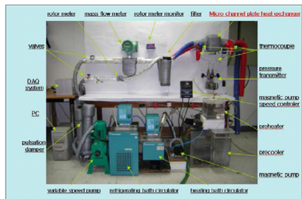
Fig. 1 The diagram of experimental apparatus for the micro plated heat exchanger.
