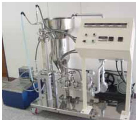
Fig. 4 Photograph of tubular reactor system
