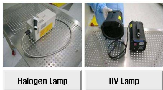
Fig. 3 Halogen and UV ramp devices for detecting foreign particles on test dummies
