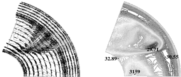
(c) Flow field and temperature contour (at z = 51.5 )
