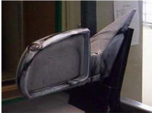
Fig. 4 Separation lines and surface vortices on side mirror visualized by the oil-film techniques.
