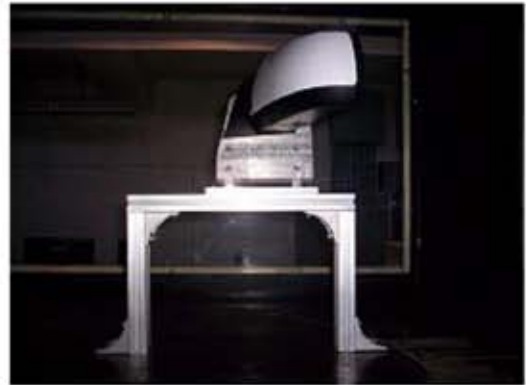
Fig. 1 Sketch of a side mirror unit on mounting zig in the wind tunnel test section.
