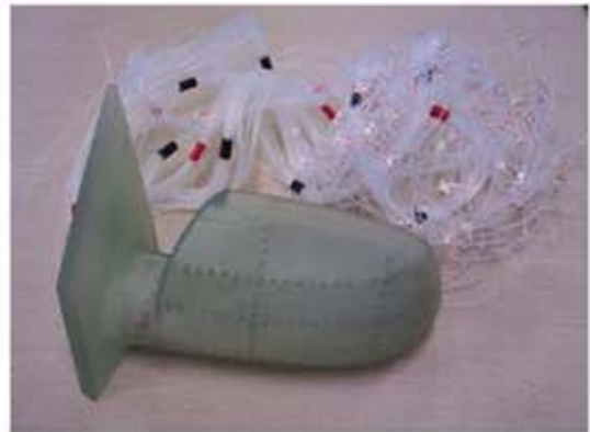
Fig. 2 RP pressure model with 100 static holes both on the mirror housing and on the mirror surface.
