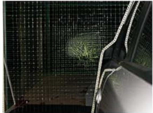
Fig. 9 Wake vortex image visualized by a tuft grid section behind the side mirror of the real scale vehicle.
