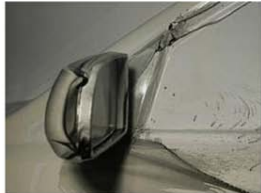
Fig. 7 Separation lines and surface vortices on side mirror mounted on the real scale vehicle, visualized by the oil-film technique.
