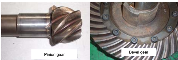
Figure 6 Damage of pinion gear surface
