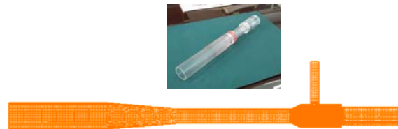
Fig. 2. The ejector model with trim cell mesh generation (inset: real ejector).
