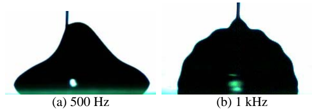
Fig. 4 Droplet oscillation for different frequencies ( V_{rms}=120 V)
