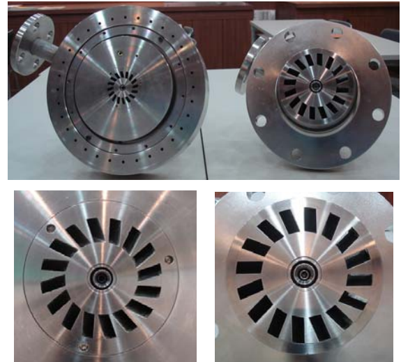
Fig. 3 GE7EA gas turbine fuel nozzle(right) and model fuel nozzle for ambient pressure experiment(left)
