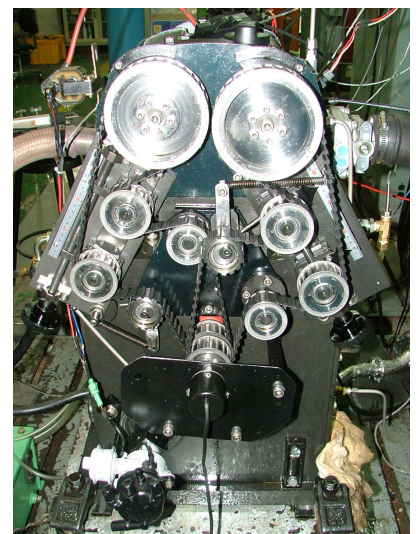
Fig. 1 Schematic diagram and photograph of experimental hydrogen fueled engine with MCVVT system
