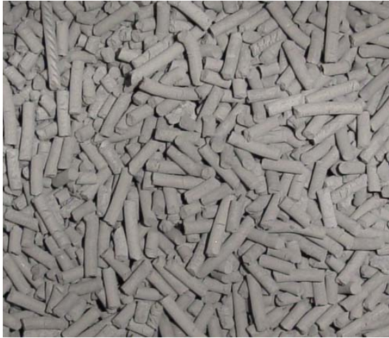
Fig. 4 Cemented tungsten carbide feedstock manufactured by the presented approach
