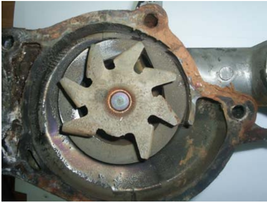
Fig. 1 Damaged impeller blades
