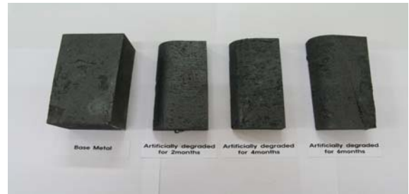
Fig. 1 CF8A steel artificially degraded at high temperature
