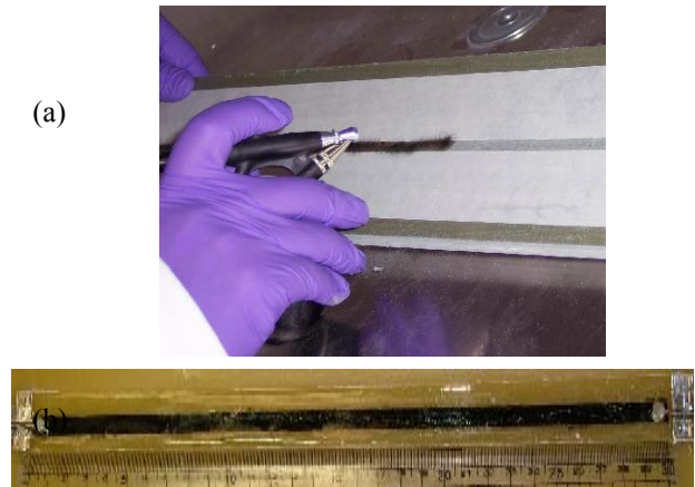
Fig. 1 Fabrication of CNT/PMMA composite electrodes (a) spray fabrication on a patterned bar; and (b) fabricated MWCNT/PMMA structural sensor sprayed on a glass fiber beam (5 wt % MWCNT, 330 x 5 x 0.08 mm, R=117.03 k, C=14.7 pF).
