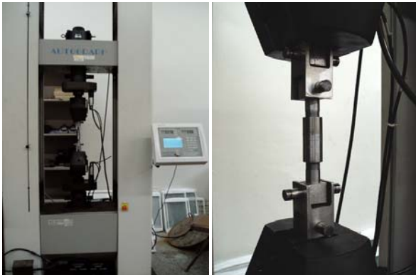
Fig. 2 Experimental setup for evaluating bond strength(SHIMADZU AG-25TG)
