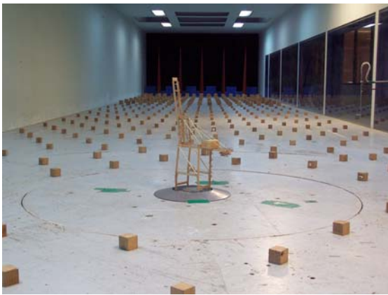
Fig. 4 The container crane model for wind tunnel test
